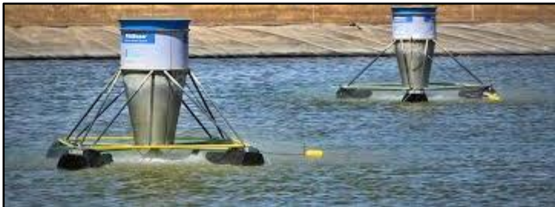
Figure 2: Sprayer-less evaporators mobilised to a major Pilbara mine site
